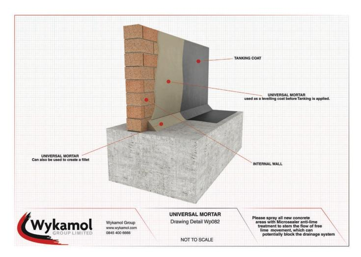
If you are using tanking slurry on a brick or stone built wall please make sure you use Wykamol universal mortar first as a levelling coat for preparation as in diagram.
